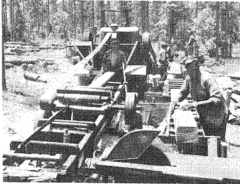
Example A—Long Jack Shaft Allows Use of Straight Belt
