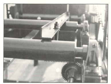
Gear and Rack Adjustable Straight Edge Fully Closed Front With Kick Back Fingers Saw Pointer Shows Location of Moveable Saw
