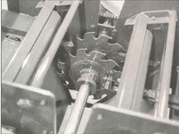
Flat-Belt Feed Roll Drive Off Arbor All Guards Over Moving Parts Factory Mounted Moving Parts Visible Through Guards for Easy Maintenance Heavy Steel Top Cover Hinges Open for Easy Service of Saws Key is Anchored to Shaft and Is Full Length of Shaft Steel Machine Flutted Feed Rolls
