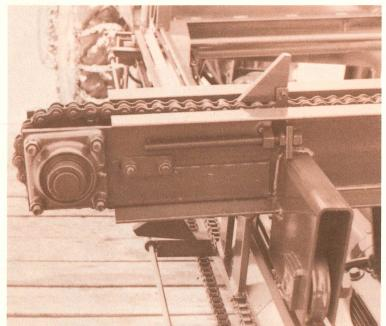
Motors and Saws Mounted on Traveling Lumber Feed Chain Unit. Entire Unit Travels on 4 Guide Wheels Mounted in Frame. Heavy Channel Chain Guides. Inserted Tooth Saws for Easy Maintenance.
