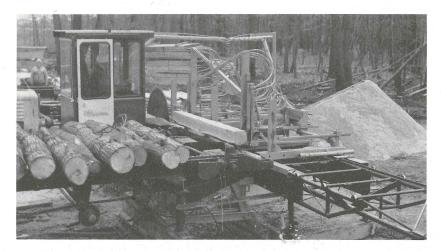
The Hydraulic Lumber Harvester is a unique portable machine. It is designed to transport to a logging site for total or partial processing of logs into lumber.
