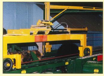
Exact 90° rotation results in square cants and lumber—log after log, day after day. End dogging unit provides positive clamping and holding of logs. The end dogger/rotator also aids in positioning logs.
